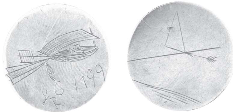
Figure 1.5 The silver disk on which Cayley engraved his concept for a fixed-wing aircraft, the first in history, in 1799. The reverse side of the disk shows the resultant aerodynamic force on a wing resolved into lift and drag components, indicating Cayley's full understanding of the function of a fixed wing. The disk is presently in the Science Museum in London.
